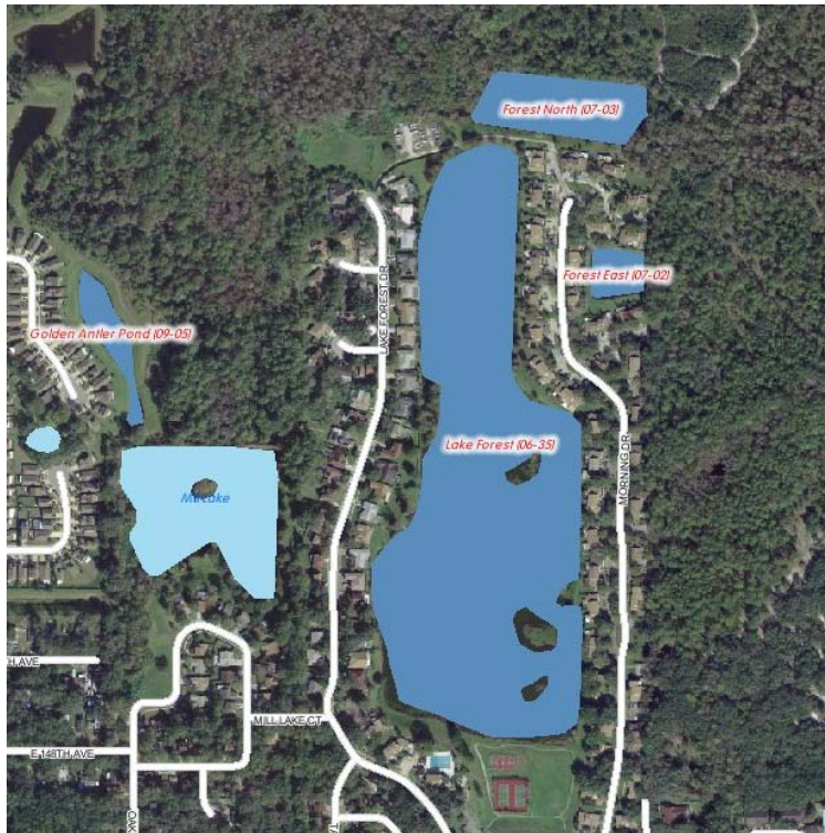
Figure 3. The Lake Forest pond system is a flow through system that takes water primarily from the Cypress Creek watershed and delivers that water back to Cypress Creek.
