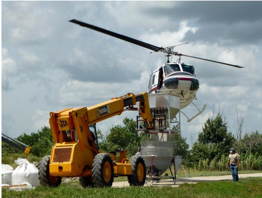
Figure 3. Loading a 909 kg bag of alum into the calibrated application bucket. The helicopter hovered over the bucket while it was being loaded!
